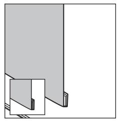
3.) Fold the fabric once over the Hem Bar Strip wrapping the Strip inside of the fabric. Fold once again to create a thick enough wrap of fabric that will be larger than the top slit opening of the Hem Bar.
