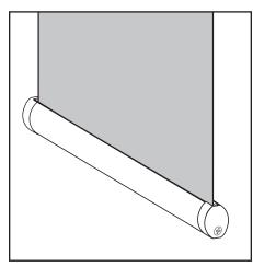
6.) Slide on the end caps and attached with the screws provided.
