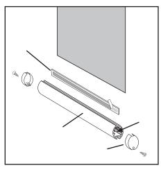
1.) Fabric should first be attached to the tube. Cut the External Hem Bar Strip and the External Bar to the same width of the fabric.
