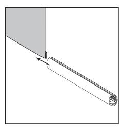
4.) Slide the External Hem Bar over the folded fabric wrapped Hem Bar Strip. Make sure the wrapped Hem Bar Strip is inside the channel and that the wrapped Hem Bar Strip is large enough so it can't be pulled out vertically from the Hem Bar.
