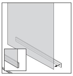
2.) Take the Hem Bar Strip and peel off the protective cover to expose the sticky tape. Apply the hem bar strip, level, to the bottom edge of your fabric.
