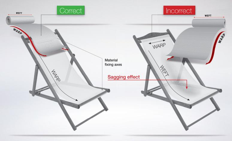
• **Correct warp and weft sense:** No problem, the tension remains perfect, no sagging. • **Incorrect warp and weft sense:** Sagging effect could appear.
