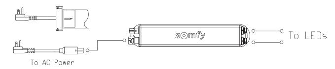
**Example 2:** The receiver and motor are plugged separately for power, each directly into the power outlet.
