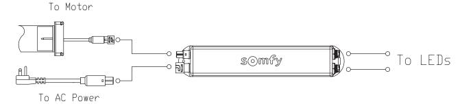
Example 1: Utilizing the Sunea® motor the receiver is plugged into the motor and both are powered from the same source via Sunea® power cord.
